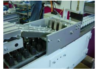
Gasflaming station for the cap surface pretreatment. With the use of the gasflame the advance of the ink gets increased.
