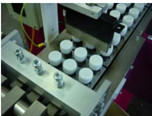
Gasflaming station for the cap surface pretreatment. With the use of the gasflame the advance of the ink gets increased.
